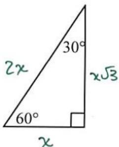
$$\begin{aligned} a^2 + x^2 &= (2x)^2 \\ a^2 + x^2 &= 4x^2 \\ a^2 &= 3x^2 \\ a &= \sqrt{3x^2} \\ a &= x\sqrt{3} \end{aligned}$$
