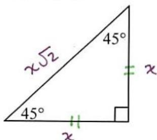
$$\begin{aligned} x^2 + x^2 &= c^2 \\ 2x^2 &= c^2 \\ \sqrt{2x^2} &= c \\ x\sqrt{2} &= c \end{aligned}$$
